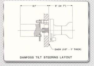
Manufactured out of 316 stainless steel, this state-of-the-art helm offers 50° of effortless tilt (25° up / 25° down). This is the original patented design with several upgrades. You will not find a stronger, more durable unit anywhere on the market. It comes with everything necessary to engage with Outboard Danfoss, SeaStar, U Flex, Char Lynn hydraulic, Mercury JPO and more and includes mounting for a new Zeiger, Isotta, Dino and Momo steering wheels.
